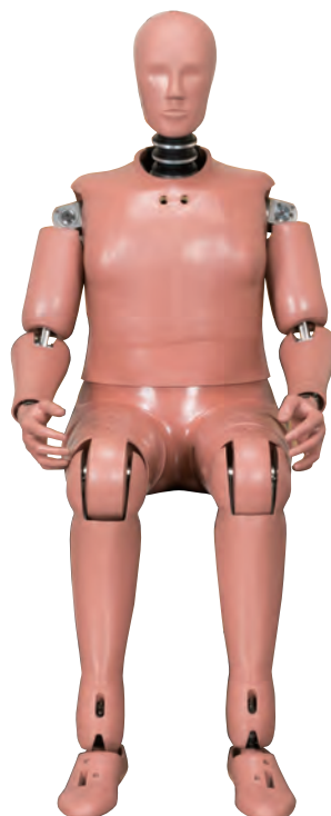
Light weight Hybrid-III 95th Percentile Male Dummy (30 kg)
